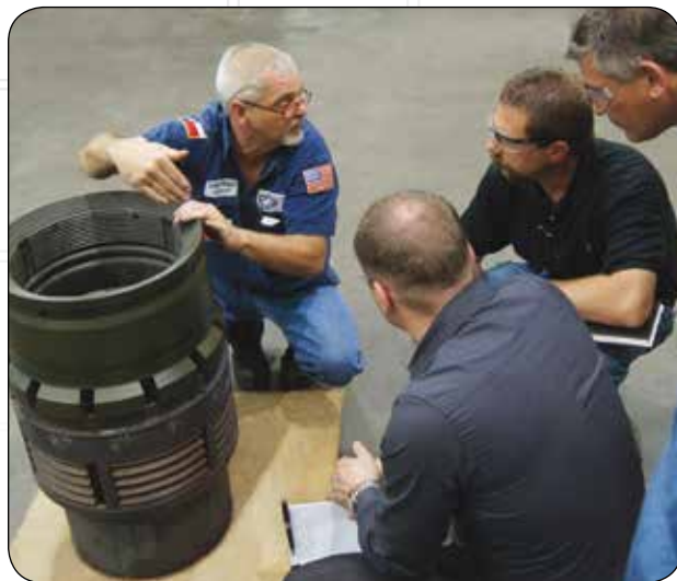
Inspection of SS-15 BigBore II-H casing hanger
