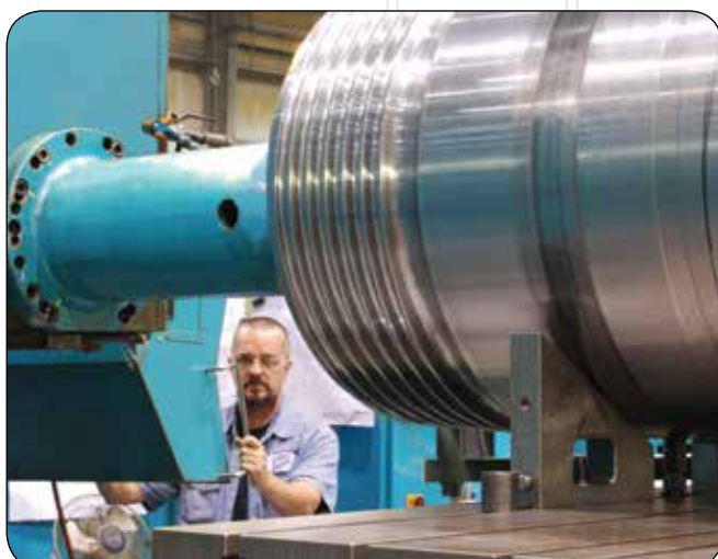
Machining of the SS-20 BigBore II-H wellhead with SDX locking profile
